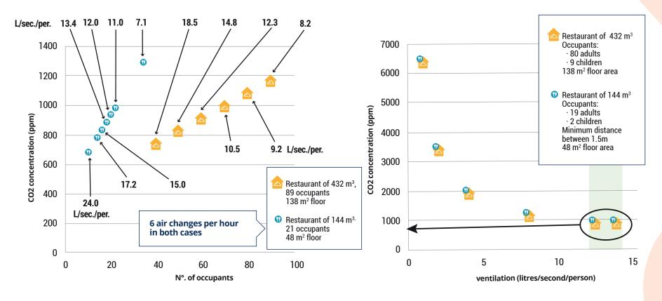
For the same dining room volume, if the number of occupants (persons) increases, the air change rate per hour should be increased to reach the recommended per person ventilation rate and avoid increase of the CO2 level.
